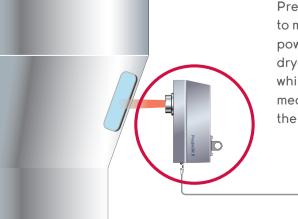
PrediktIR II can be installed to measure moisture in powders in a fluid bed dryer through a sight glass, while ensuring that the measurement area is below the powder line.
