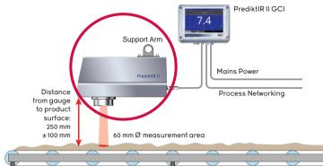
PrediktIR II measures over a 60 mm diameter standard beam patch size. It is suspended over the process line at a distance of 250 mm from the mean product height and tolerates product height fluctuations of ±100 mm.
