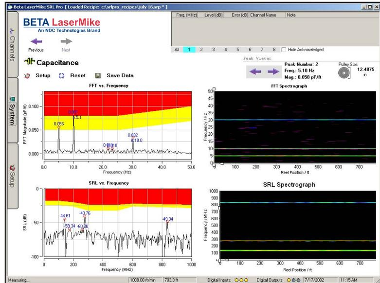
The Beta LaserMike SRL Pro™ is the first reliable predictive analysis tool designed specifically to find Structural Return Loss (SRL) problems and identify potential causes of these problems on Datacom insulation lines in real time before they cost you time and money.
