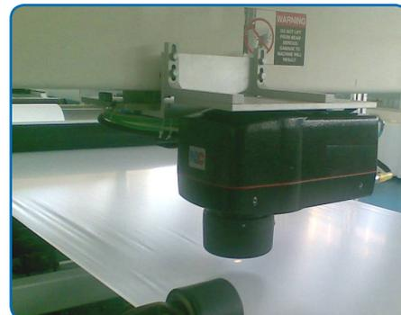
NDC's FG710S Infrared Sensor measuring the true thickness of LIB separator film
